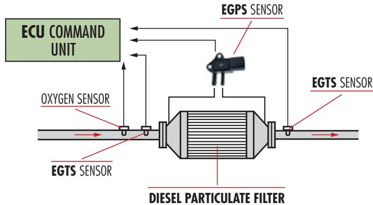
The EGPS is found in Diesel Particulate Filter Systems with additive (FAP) and without additive (DPF).
